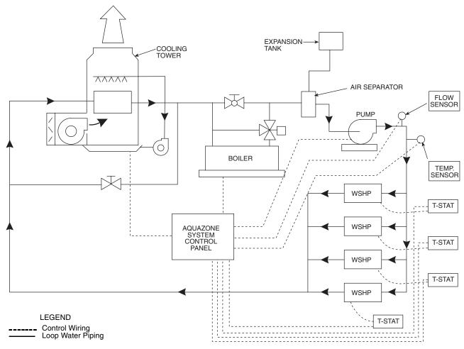
Fig. 2 — Typical Stand-Alone WSHP System
